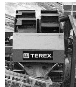
Rubber lined chute on discharge
