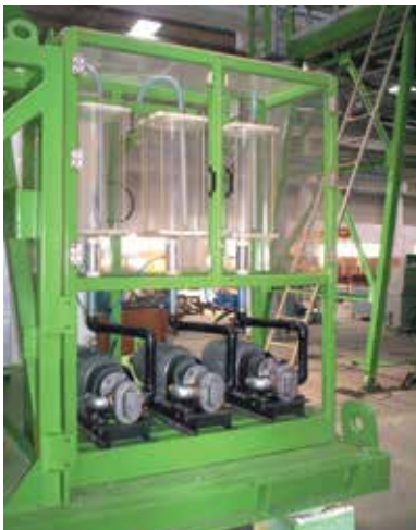
Admixture weighing system for chemical additives.
