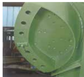
Large-dimensional mixer discharge with hydraulically actuated sliding gate for fast discharging.
