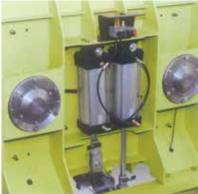
The pneumatic discharge gate operation
