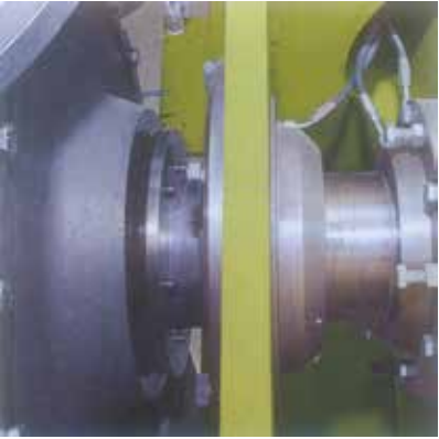
Separataed : sealing and bearing.
