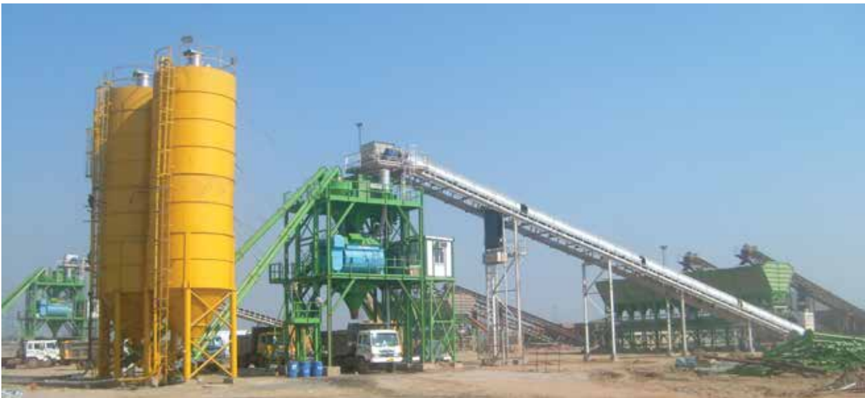
The H6 plant at Dankur that set record in PQC production (5050 cu.m in 1 day)
