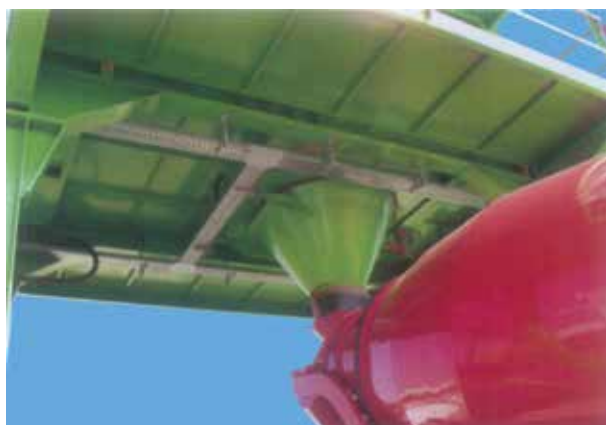
The mixer discharge for filling truck mixers.
