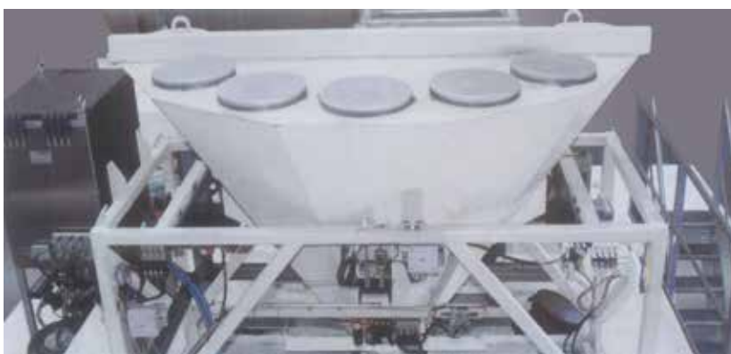
The cement weighing system for up to seven types of cement.
