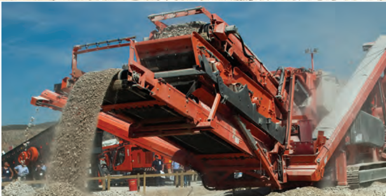
Optional hanging screen can provide a 1, 2 or 3 way product split
