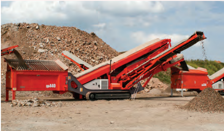
Sandvik patented Doublescreen for higher accuracy and productivity
